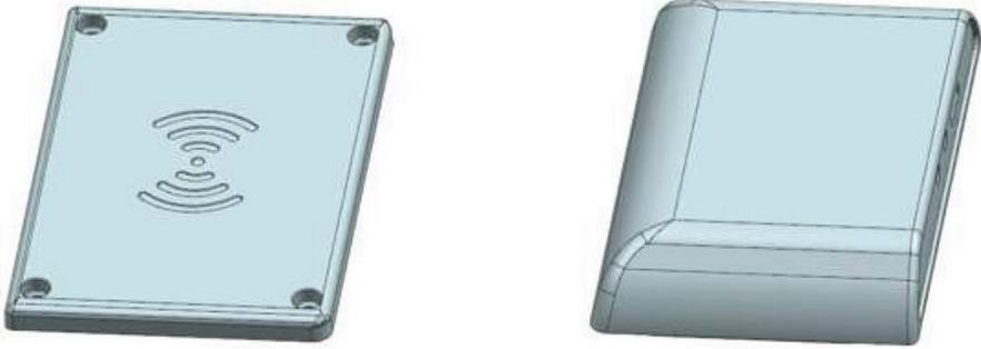
**Figure 3.16** Designed housing. Initial design.
