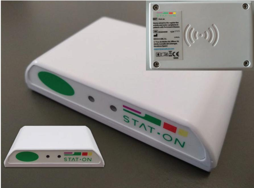
**Figure 3.22** Final industrialized enclosure of the STAT-ON™ device.
