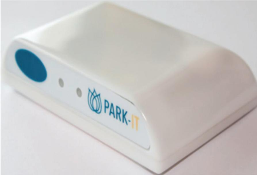
**Figure 2.1** Redesigned PARK-IT wearable prototype.
