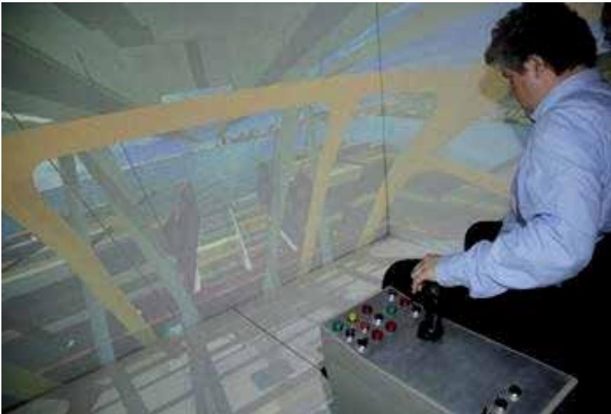
The simulators work with a replica of the cabin with all the active, integrated controls of a visualization system in digital CAVE. [Image: COPPE/UFRJ]. Extracted from <http://www.inovacaotecnologica.with.br/noticias/noticia.php?artigo=simulador-portuario>
